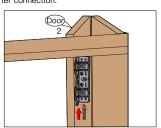
3.3 Connect the down roller of door 2 with the roller on down rail which is close to the fixed door.
