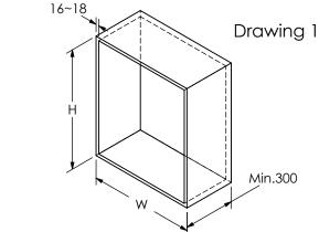
(2) Drill the side-board of the cabinet then fix accessory "A", "B" one by by one as the following drawings.
