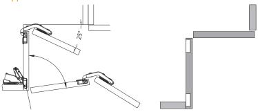
Use with 165 degree opening angle hinge
