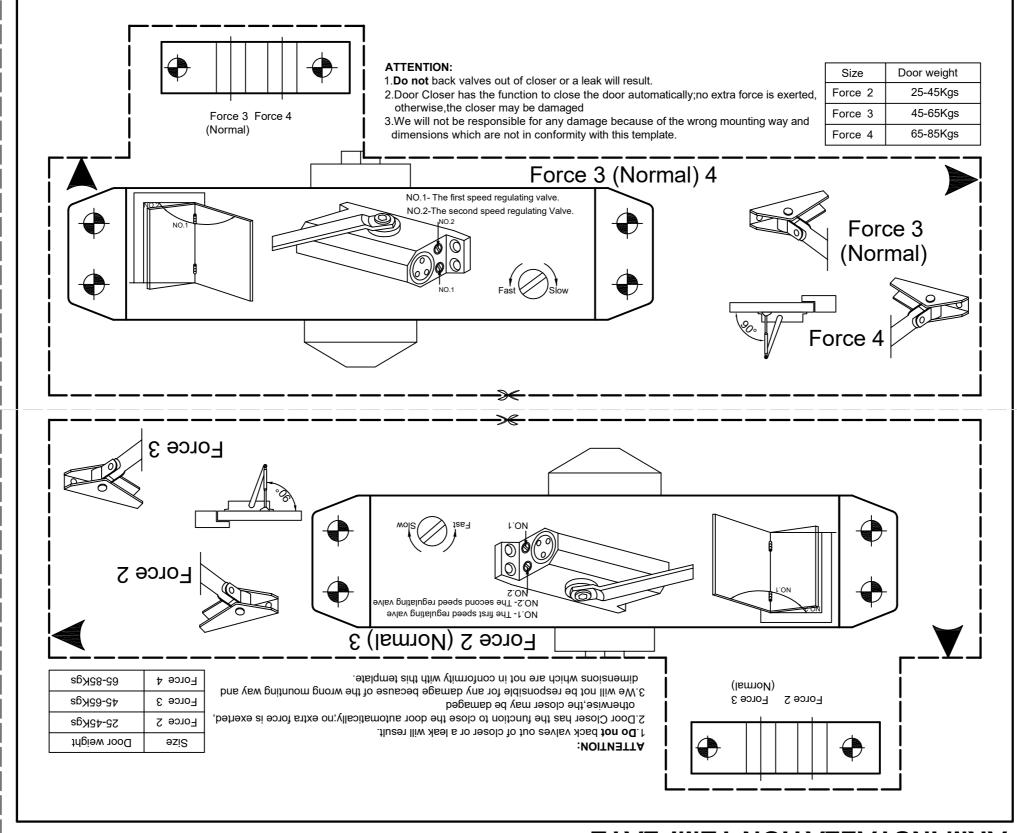
IMUNDEX OVERHEAD DOOR CLOSER WITH HOLD OPEN ARM INSTALLATION TEMPLATE
